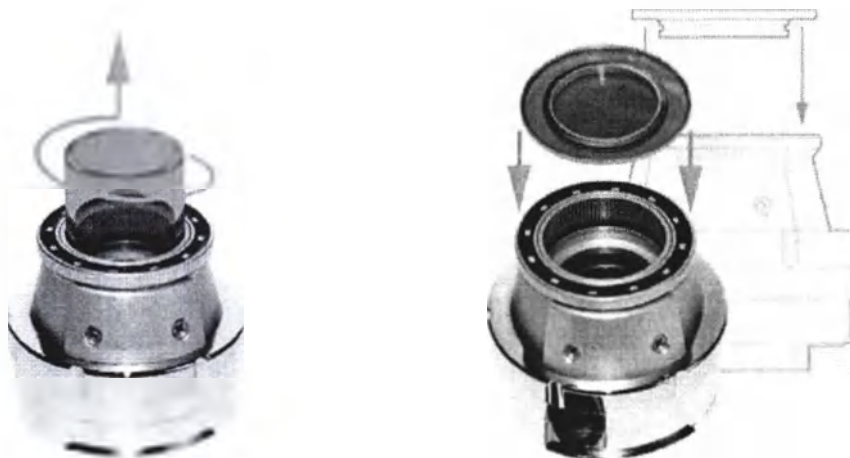
Image 19. Attaching glass tubes and polarizing filter to the dermoscopy lens.
