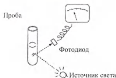
Figure 2-1. Scheme of the light flux of the coagulation process.
