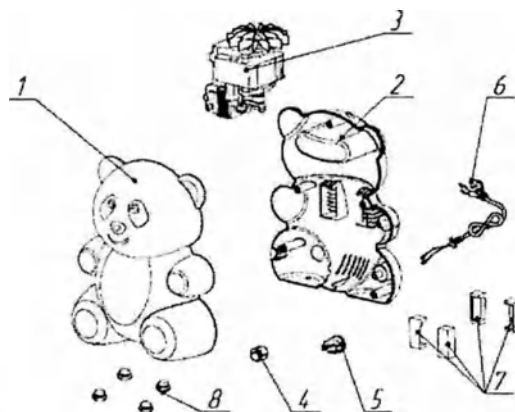
Fig. 2.28 Compressor circuit in the product version A500LW12 1 - front part of the body; 2 - back of the case; 3 - the engine; 4 - the filter cover; 5 - the switch; 6 - power cable; 7 - a support of the engine; 8 - the foot of the compressor.
