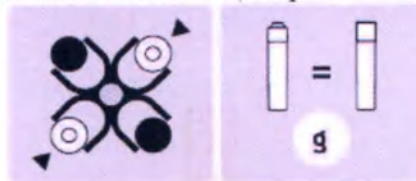
Figure 5: the right position of tubes
