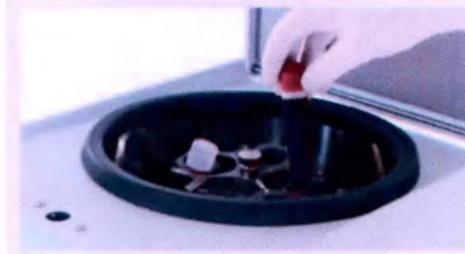
Figure 4: Positioning of the tube in DUOGRAFTER II with the counterweight tube
