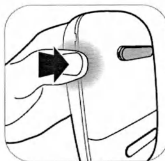
3. Open the motor unit by pressing at the sides of the device.
