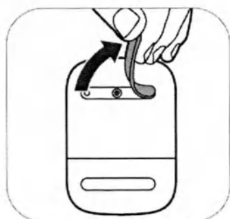
1. Remove the rubber gasket from the bottom of the motor unit.
