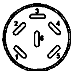
Pin Arrangement in DIN Socket for analog output
