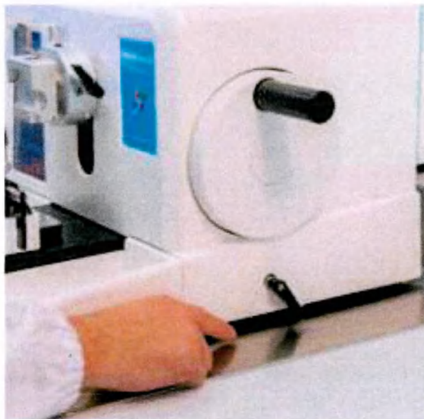
LEVER AWAY: HANDWHEEL UNLOCKED
