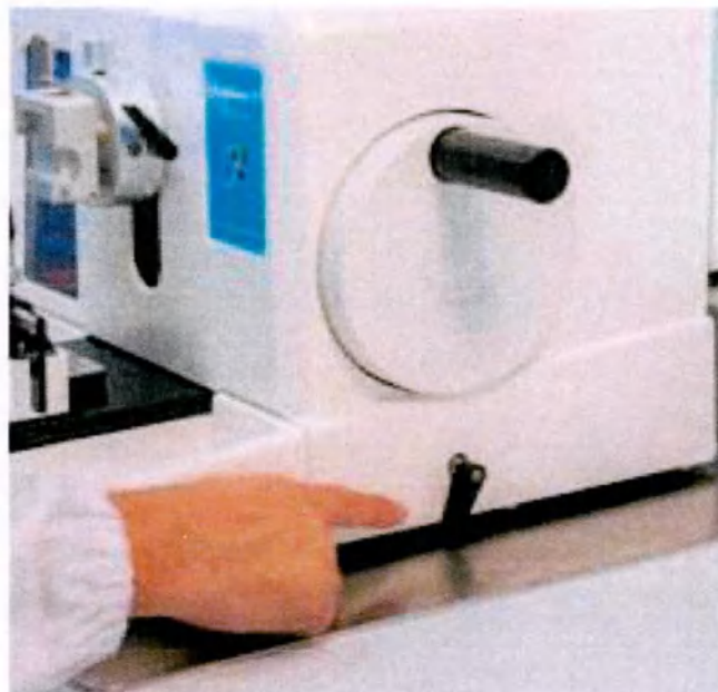
LEVA NEAR: HANDWHEEL LOCKED
