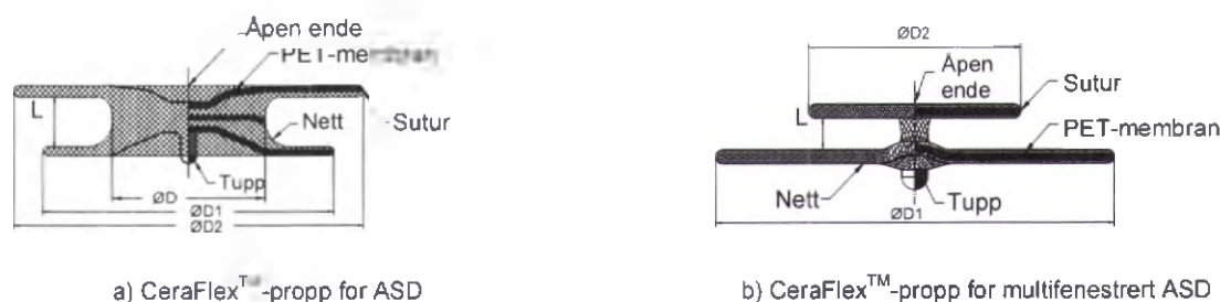
Figur 4. CeraFlex™-propper for ASD
