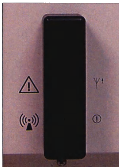
Figure 11, Example of the wireless antenna located on the device rear panel
