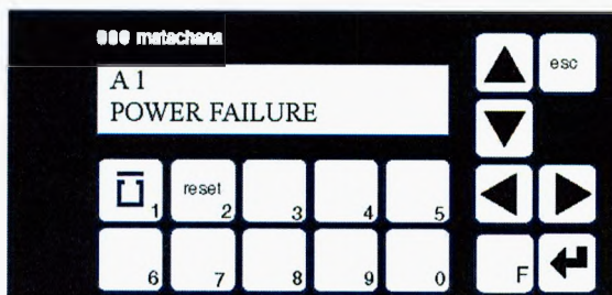
Figure 2.6: Screen 2.3. Active alarms.
