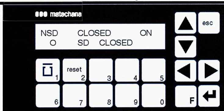
Figure 3.2: Sterile area control panel. Door status.
