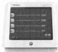
Figure 2. Representative image of the Symplcity G3™ renal denervation RF generator displaying the impedance monitoring screen
