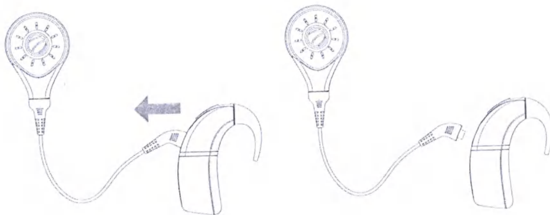
Figure 13. Removing the Transmitting Coil and the Signal Processing Unit
