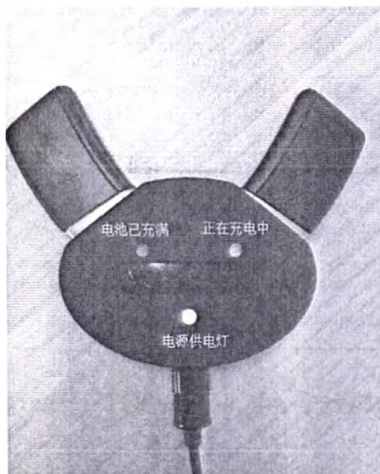
Figure 17. Charging method of the BTE rechargeable battery compartment
