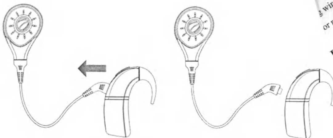
Figure 13. Removing the Transmitting Coil and the Signal Processing Unit
