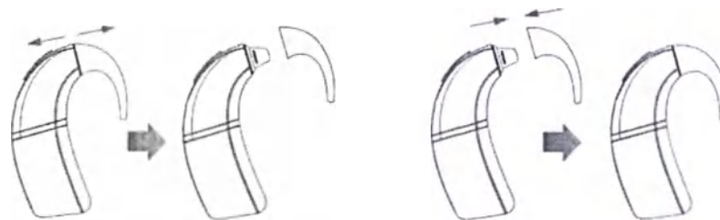
Figure 11. Method for Replacing the BTE Hook
