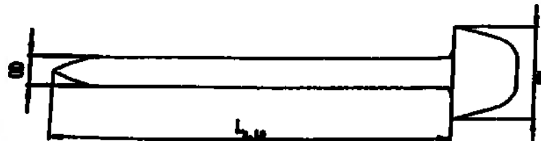
Figure 2b) – the shape of the working part of the stylet is a conical needle without edges (OD – outer diameter of the stylet, L_{s,tp} – length of the rod of the stylet, D_s – maximum diameter of the stylet tip) – for the following versions: NPCS-70-1-3, NPCM-70-1-3, NTCS-70-1-3, IIC-70-1-3, IC-50-1-3, IC-70-1-3, IC-90-1-3 ;
