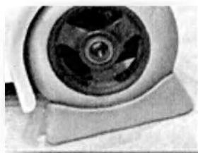
Figure 3. External view of the roller stopper
