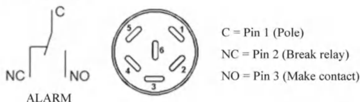
Figure: Zero-voltage contacts circuit diagram and pin allocation of DIN socket (13)
