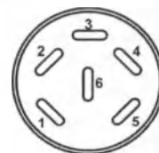
Figure: Pin configuration of the DIN socket (3) on the chamber rear
