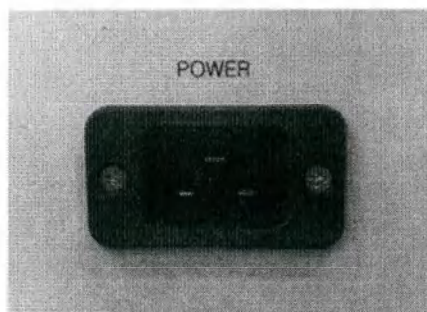
Figure 3. Power in put terminal - power cord connector
