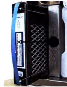
Figure 67. Removing the filter
