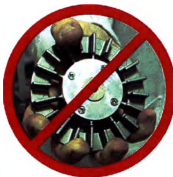
Figure 65. Stirrer handling—correct (left) and incorrect (right)
