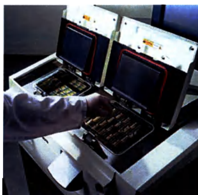
Figure 7. Placing a basket into a retort
