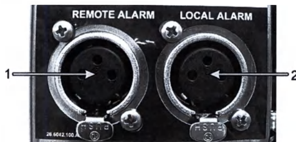
Figure 21. Remote alarm (1) and local alarm (2) connectors
