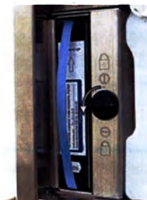
Figure 69. Locking the filter
