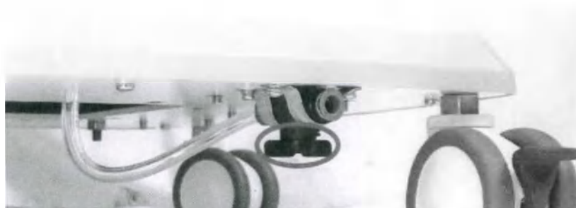
Figure 27. Air compressor condensate remove
