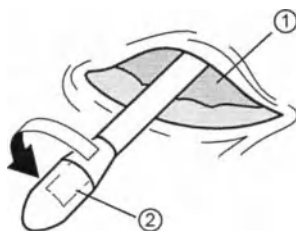
Figure 3. Removing the tip from the tunneling rod.
