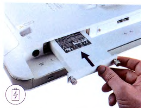
11. Slide the battery into the battery slot and tighten the thumb screws
