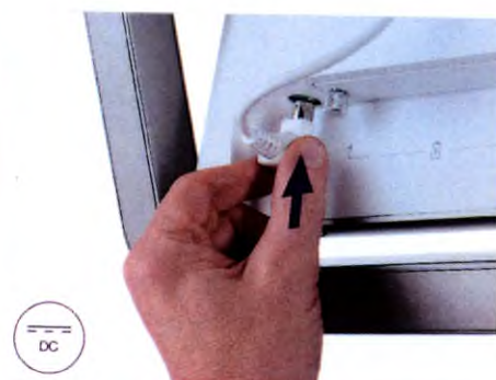
14. Attach the power cable to the port labeled DC
