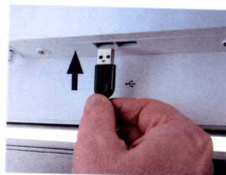
23. Plug in the webcam to the USB port at the bottom of the HD screen
