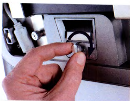
13. Turn the scanner around and tighten the thumb screw to secure the HD screen
