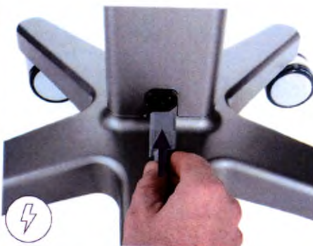
19. Attach the power cable on the bottom of the wheel stand
