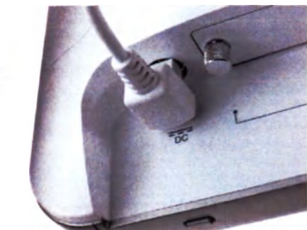
15. Power cable inserted
