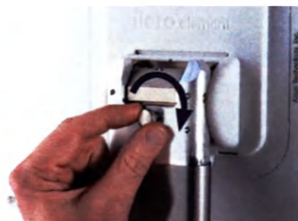
6. Turn the scanner around and tighten thumb screw to secure HD screen
