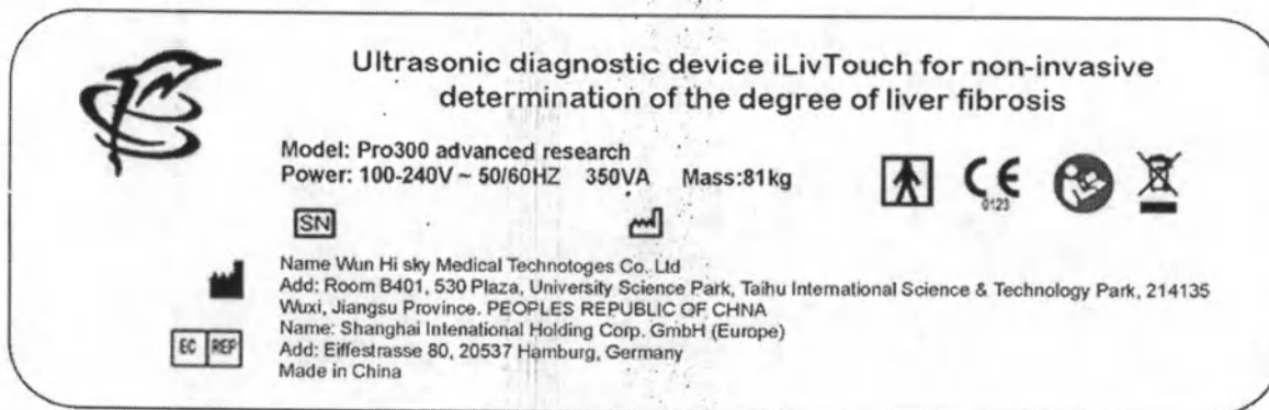
Fig. 11-2 - Marking of the plate of the main unit model Pro3000 advanced search on the back of the machine.
