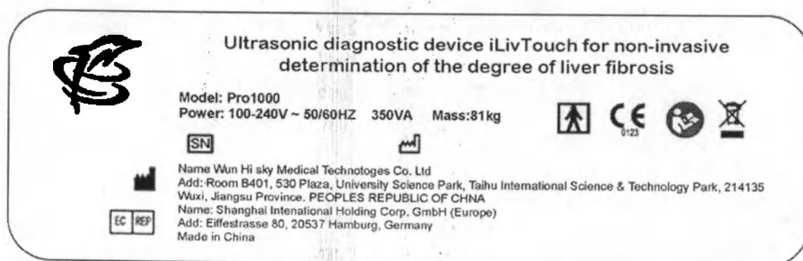
Fig. 11-1 - Marking of the plate of the main unit model Pro1000 on the back of the machine.
