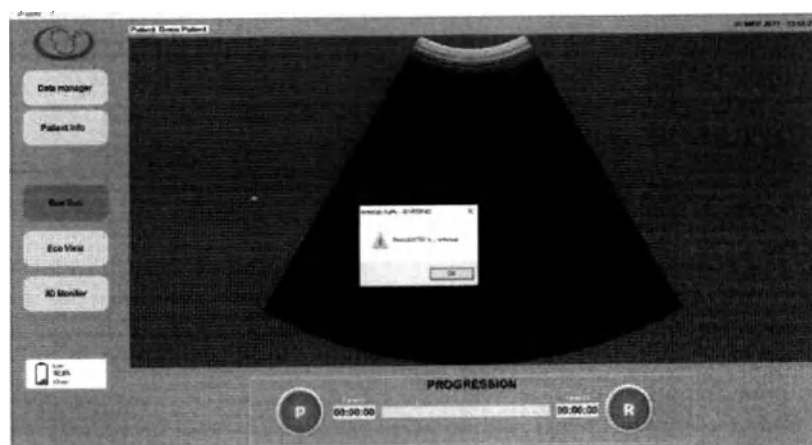
Figure 36. The alert window «Press ENTER to continue» appears to indicate that the system is in FREEZE mode. To continue scanning and resume the activity of the system, click on "OK".
