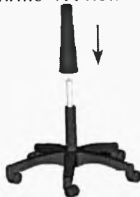
Figure III-3 Installation of decoration cover of air spring
