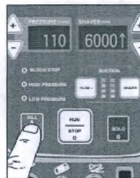
Fig 7. Press FILL Chamber Pad to Prime Pump
