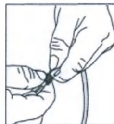
Fig 8. Remove Blue Caps from Intermediary and Inflow Tubing and Connect Intermediary Tube
