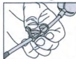
Fig 9. Open Clamp under Pressure Chamber
