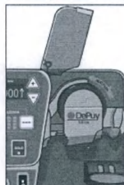
Fig 10. Position Outflow Tubing on Pump Roller
