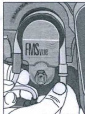
Fig 3. Position the Green Autolock on the Pump
