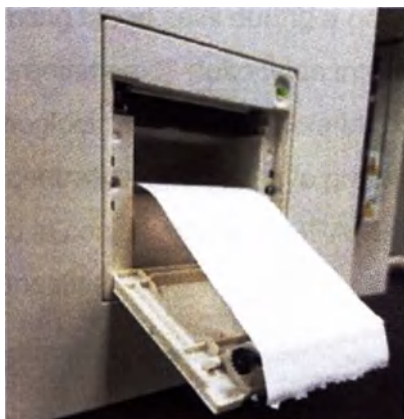
Figure 2-9 Installing thermal paper (2)
