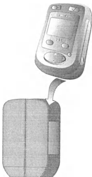
Figure 2.20 Insert the patient programmer into the case.
