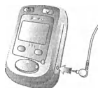
Figure 2.24 Insert the antenna plug into the antenna jack.
