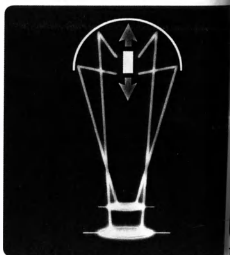
Adjustment of bulb location against reflector
