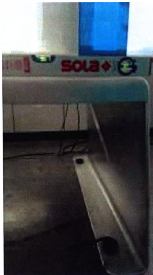
Figure 4.3 – leveling the densitometer.
