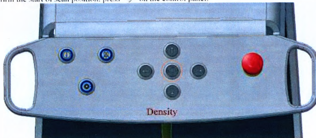
Figure 5.20 – indication of "start" buttons on control panel
