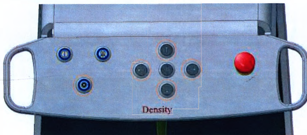
Figure 5.19 – Density control panel: arrows and laser pointer
