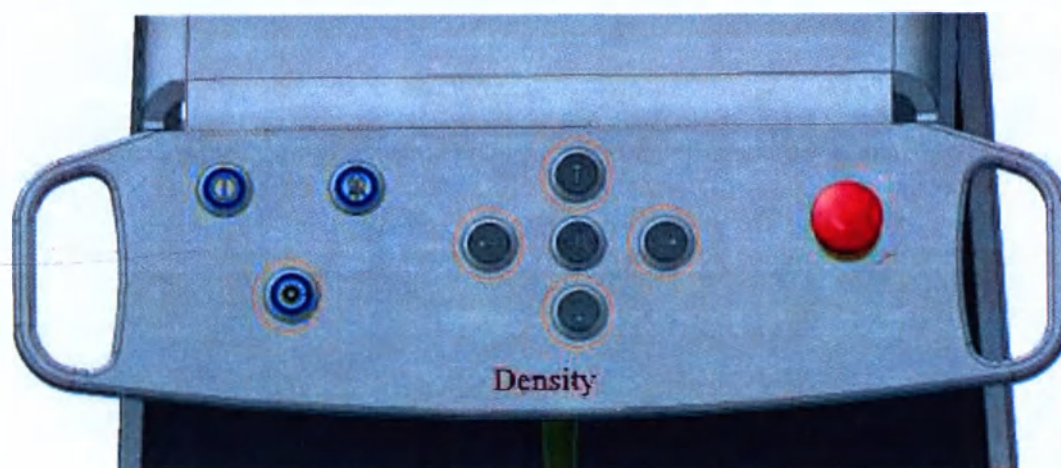
Figure 5.19 Density control panel: arrows and laser pointer
