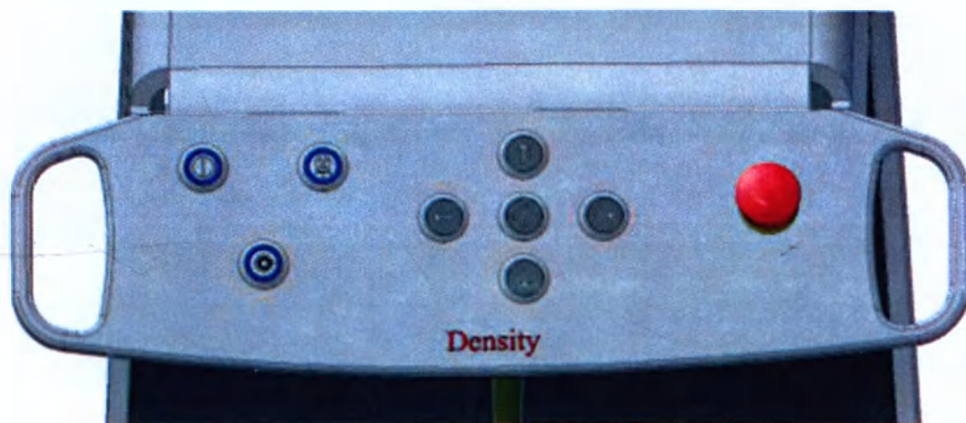
Figure 5.19 Density control panel: arrows and laser pointer
