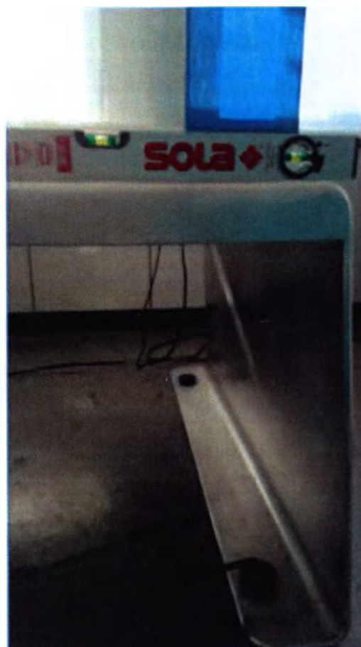
Figure 4.3 – leveling the densitometer.
