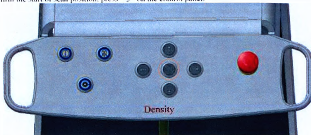
Figure 5.20 – indication of "start" buttons on control panel
