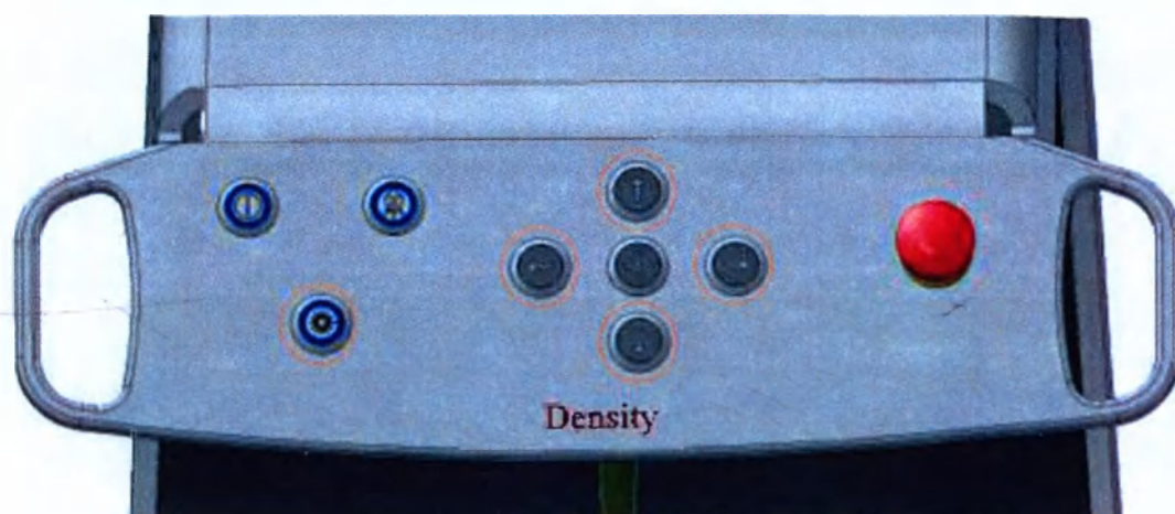
Figure 5.19 Density control panel: arrows and laser pointer
