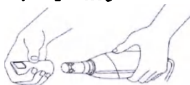
Figure 1 Handheld TRIOS® intraoral scanner (with handle) Scanner obtains 3D images of the topographical characteristics of patient's teeth. Patient contact with distal end of tip. Weight = 350 g
