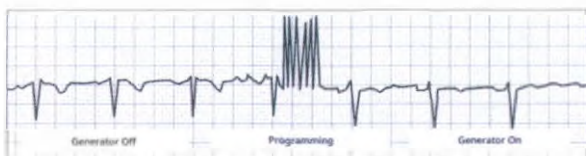
Figure 1. ECG Artifact Produced by Generator Communication
