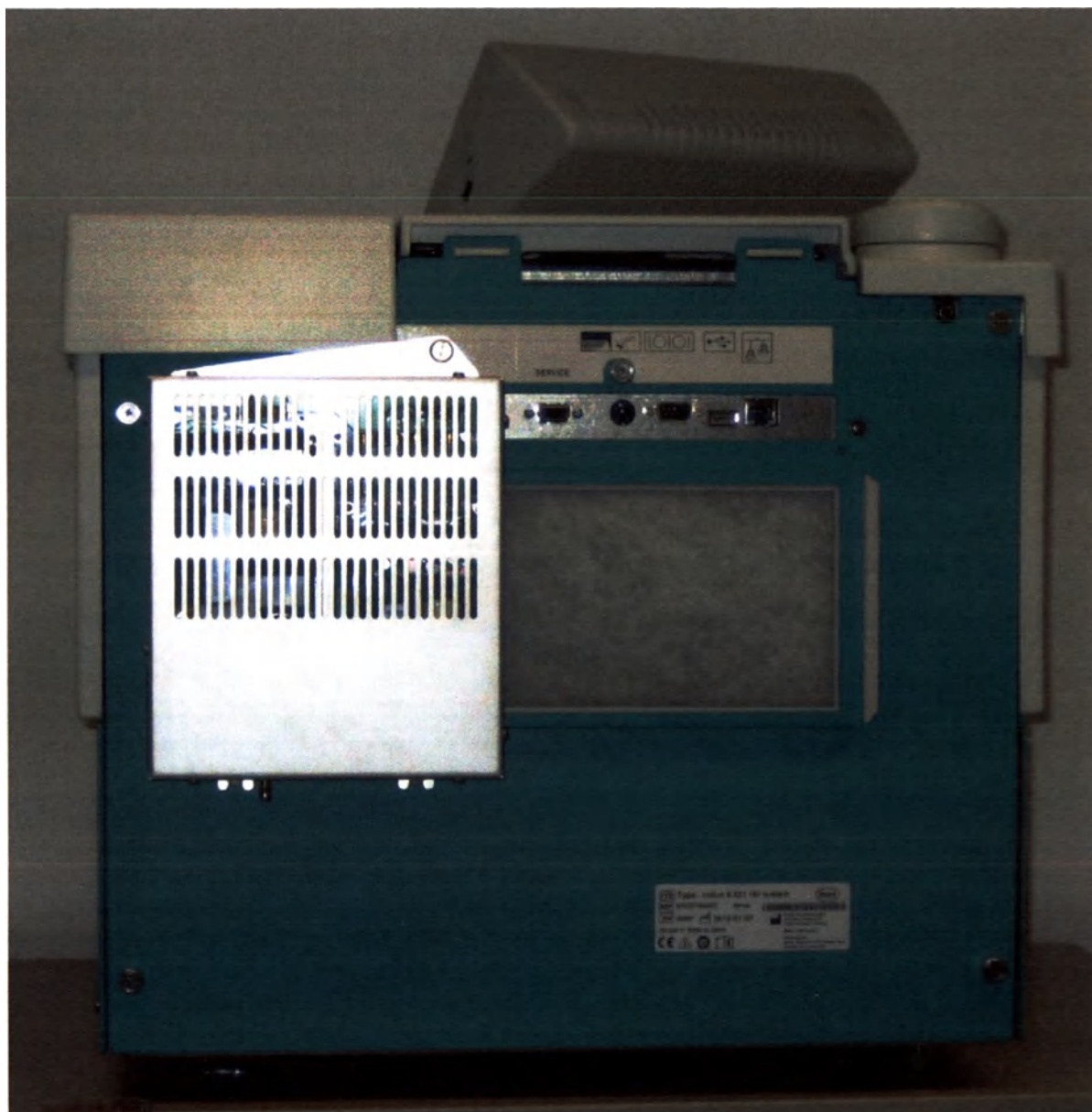
Figure 4: Rear side with replaced power supply, only minor changes therefore no change of this document necessary
