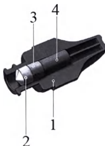
Figure 3. Diagram of the structure of the plug cap used with the Luerh connectors of the access valve
