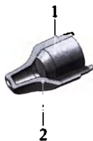
Figure 2. Diagram of the structure of the socket cap used with the Luer lock of the access valve.
