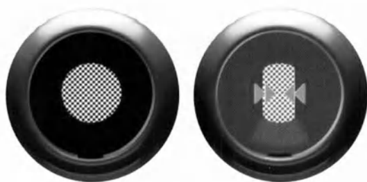
Due to the automated monitor shutter during the ERG, the EP-1000 achieves 100% Ganzfeld conditions.
