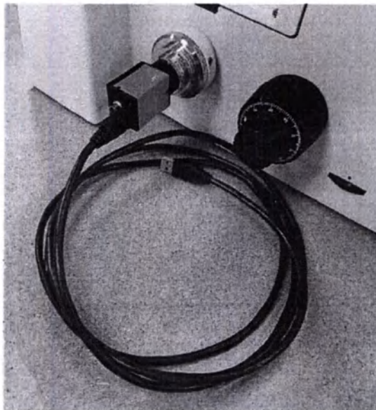
Figure 3-5: JAI Digital Camera Installation using Leica OEM C-Mount Adapter (example).
