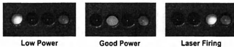
Figure 3-4: Laser Controller LED Status Bar
