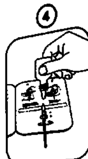
a Add 8 drops of buffer to well A b Rotate the strip, two rounds each direction
