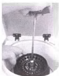
Tool for rotor with nut.
