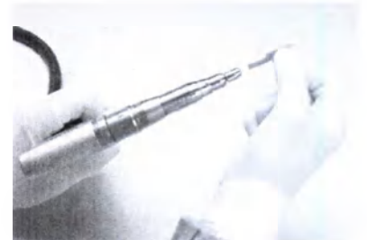
Figure 2-2. Reciprocating Saw Assembly
