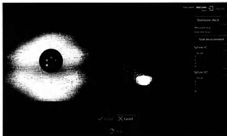
Fig. 62: Alignment: bad lenslet reflex
