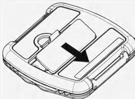
Figure 3. Removing battery cover.
