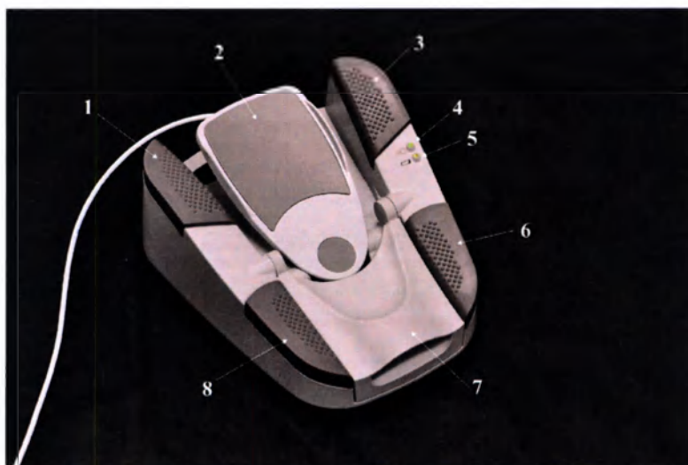
Figure 1.31. Top of Primary (Integrated) Foot Control.
