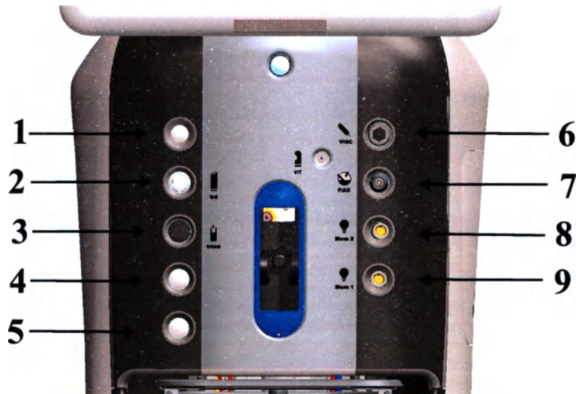
Figure 1.24. Front panel with handpiece connectors.
