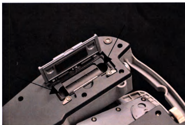
Figure 1.29. Battery compartment with recess (arrows) to facilitate battery replacement.
