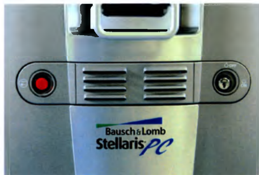
Figure 1.50. Front Panel with Emergency Laser Stop button, air vents and Key Switch.
