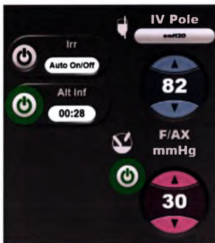
Figure 4.16. Surgical screen displays Elevated Infusion control (status ON) and timer.
