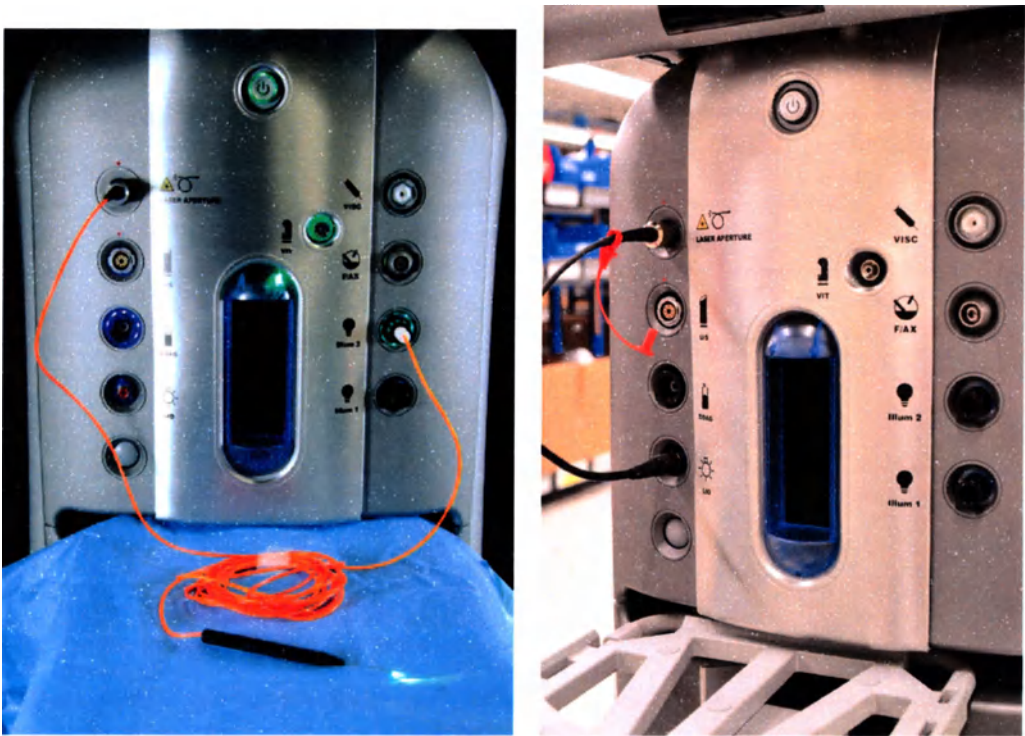
Figure 1.51. Laser handpiece (left) and LIO (right) connected to system.
