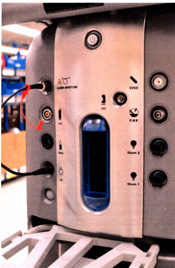
Figure 1.57. System with LIO connected.
