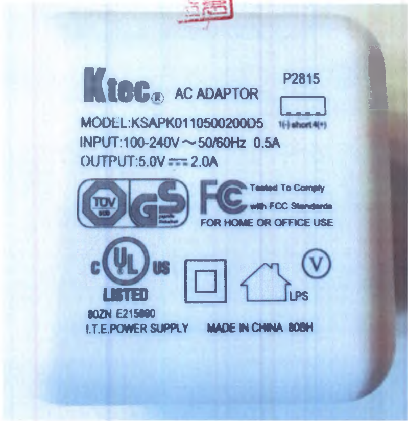
Fig. 8. DC IN Adaptor (The symbols are explained in the table 7 below).
