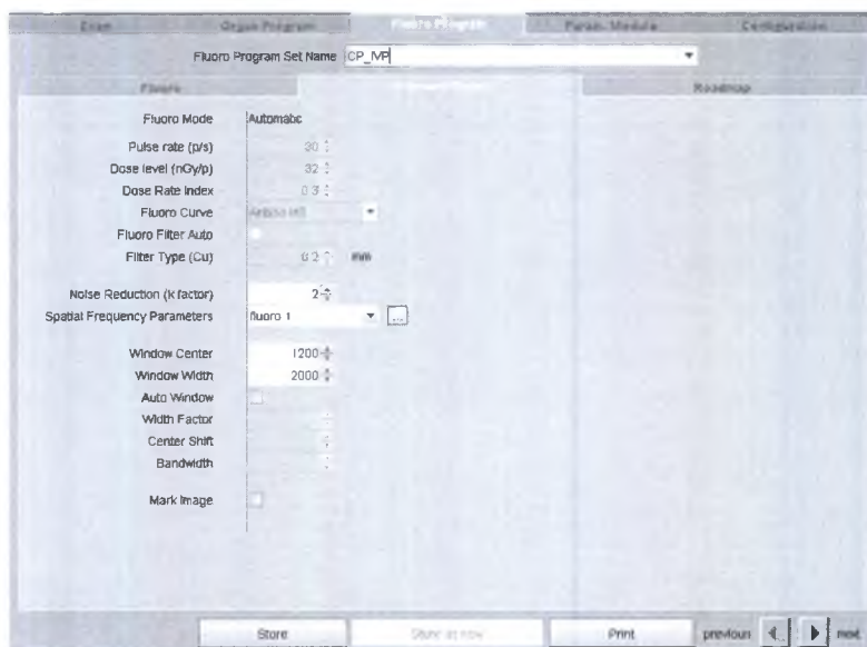
Example of Hi Speed Fluoro tab card: Parameters for high speed fluoroscopy 30 p/s
