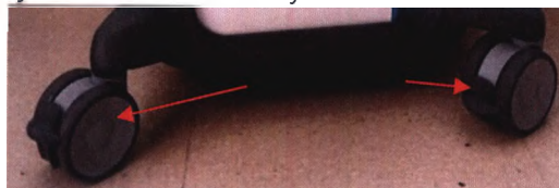
Fig. 37 The locking mechanism of the wheels. It is necessary to press the foot on the elements marked by arrows to block the movement of the rack-cart
