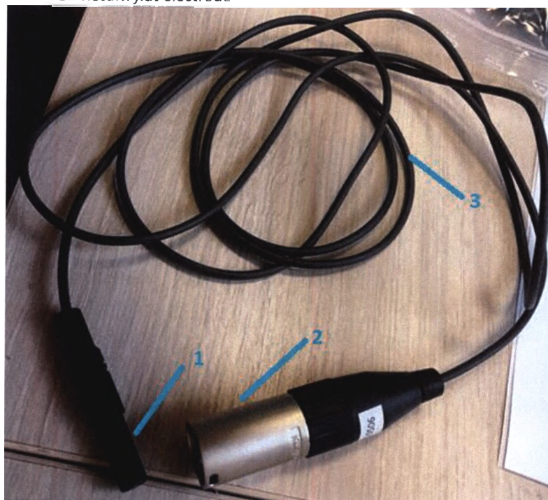
Fig. 43 The design of the cable return electrode cylindrical 1 - Connector for connecting to the electrode return cylindrical 2 - Connector for connecting to the device 3 - Wire cable electrode return cylindrical
