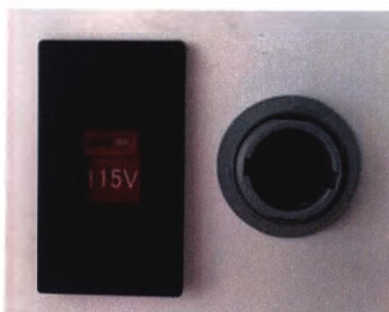
Fig. 32 Voltage switching at the rear of the trolley rack and connector for connecting the main unit with the trolley rack
