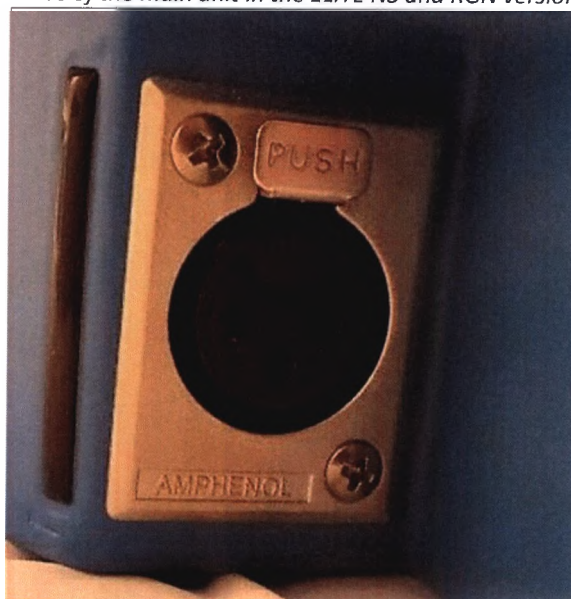
Fig. 9 Socket for connecting return flat and cylindrical electrodes. In order to remove the connector for connecting to the device from the device itself, you must press the top "PUSH" button
