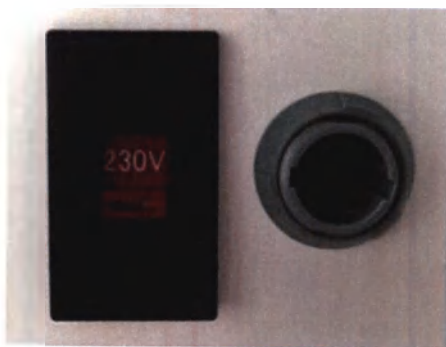
Fig. 32 Voltage switching at the rear of the trolley rack and connector for connecting the main unit with the trolley rack
