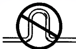
Figure 3. Coiling excess lead.
