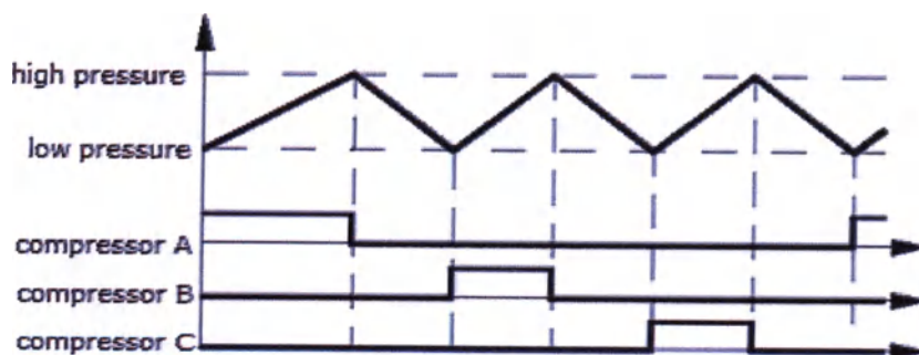
Figure 25 – Operation diagram of the screw compressors in mode «On/Off»
