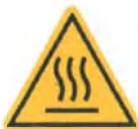
Warning label (hot surface)
