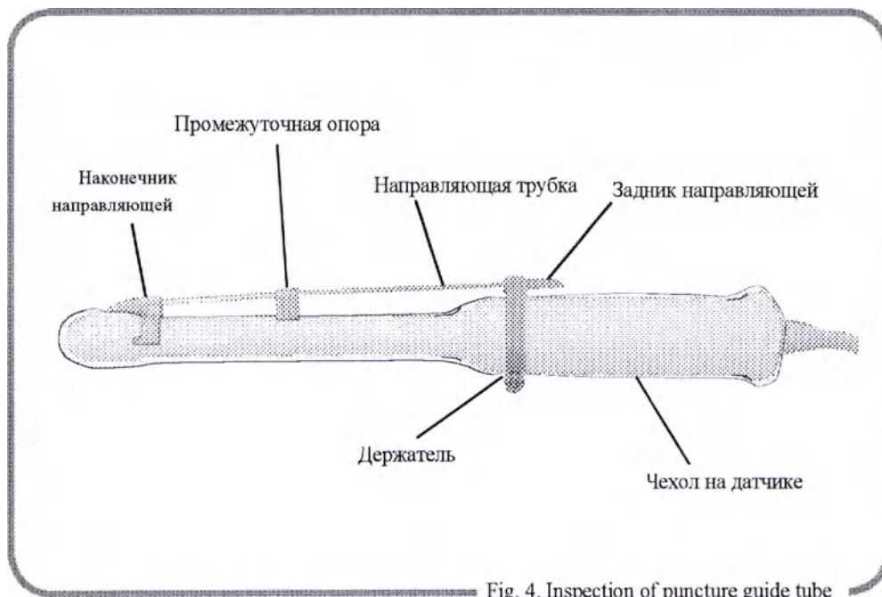
Fig. 4. Inspection of puncture guide tube
