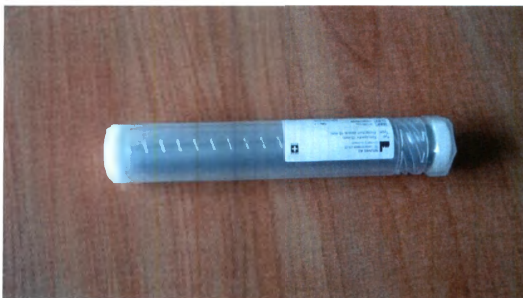
Fig. 16. Protective tube casing
